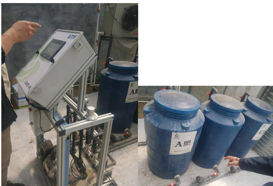
The automatic integrated fertilizer and water irrigation machine used in the greenhouse.
